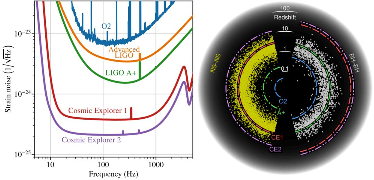
**Fig. 2:** Left: LIGO and CE strain noise for different versions of each. CE1 is scheduled for the 2030’s and CE2 for the 2040’s. Right: Response distance for LIGO implementations and CE designs superimposed on a population of 1.4–1.4  $M_{\odot}$  neutron star mergers (yellow) and 30–30  $M_{\odot}$  black hole mergers (grey). Figure from [Reitze et al. \(2019\)](#).
