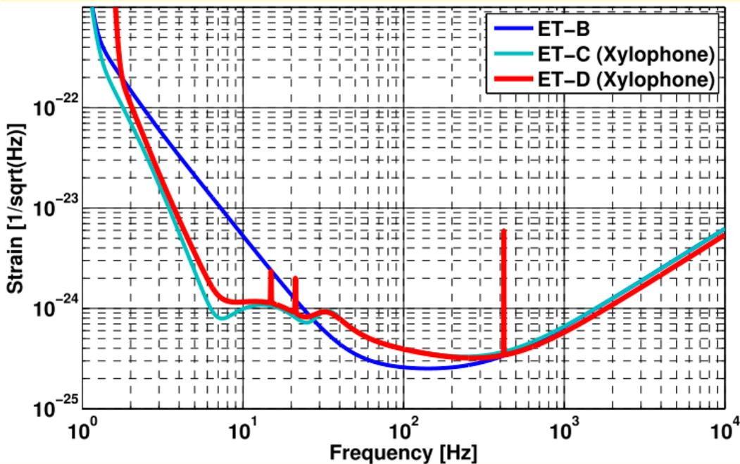
**Fig. 4:** Sensitivity of the Einstein Telescope. Figure from [European Commission \(2011\)](#). ET-B is the sensitivity when each detector is a single interferometer. ET-C is an enhanced version when each interferometer is split into two co-located interferometers: one with optimisation at high frequencies and the other at low frequencies. ET-C is the best sensitivity that is expected when all of the noise terms are included in the predicted sensitivity.
