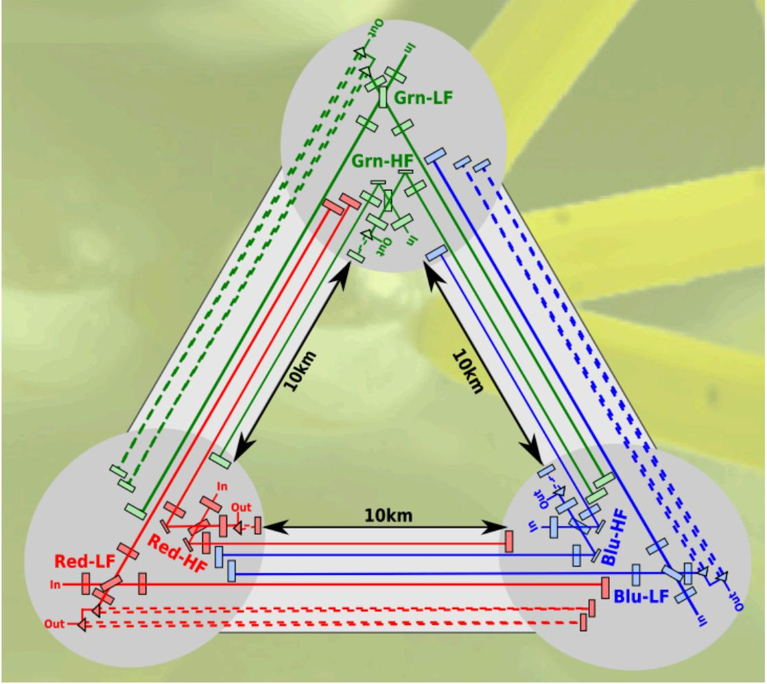
**Fig. 5:** Conceptual layout of the Einstein Telescope, Figure from [European Commission \(2011\)](#). The instrument has 3 pairs of km sized interferometers in a triangular shape. Each pair consists of a low frequency optimised detector and a high frequency optimised detector. This graphic is not to scale.
