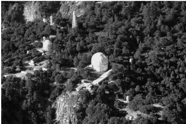
**Fig. 16.** The facilities of the CHARA (Center for High Angular Resolution Astronomy) Array together with the existing facilities of historic Mount Wilson Observatory. The Beam Synthesis Facility, an L-shaped structure of the length of a football field, can be seen close to the 2.5m telescope dome.
