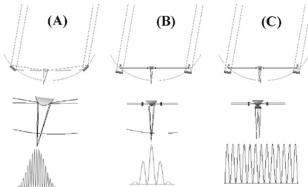
**Fig. 3.** Comparison of three different beam-combinations for an optical stellar interferometer. (A) and (B) the classical Fizeau versus Michelson beam-combinations, (C) instead of superimposing the Airy patterns from the telescopes, it is possible to use a relay lens after the beam-combiner so as to stack the two output pupils on the top of each other with a modulation depending on the output Airy discs distance.
