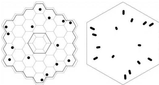
**Fig. 6.** *Desired sparse pupil (left) and the aperture mask used to generate it (right). The required pupil is shown as the set of black spots and is superimposed on a scaled version of the segmented 10m Keck primary mirror (hexagonal segments). From Tuthil et al. (2000).*
