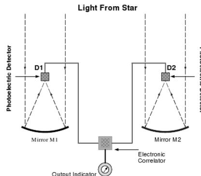
**Fig. 2.** Intensity interferometer arrangement. The interferometric signal, the degree of mutual coherence, is characterized by the degree of correlation of light intensity fluctuations observed at two different detectors.
