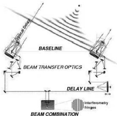
**Fig. 4.** Michelson's interferometer. The light from each aperture is carried to a common focus, combined coherently in order to detect interferometric signal (fringes). Beam transfer optics and delay lines allow it to maintain equal path length between the telescopes as the object is tracked across the sky.
