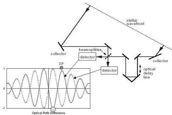
**Fig. 8.** *Nulling Interferometry Principle.* The starlight that arrives at a pair of telescopes so that a deep destructive fringe is placed across the star (making it disappear), but the light coming from a planet gets added rather than subtracted.
