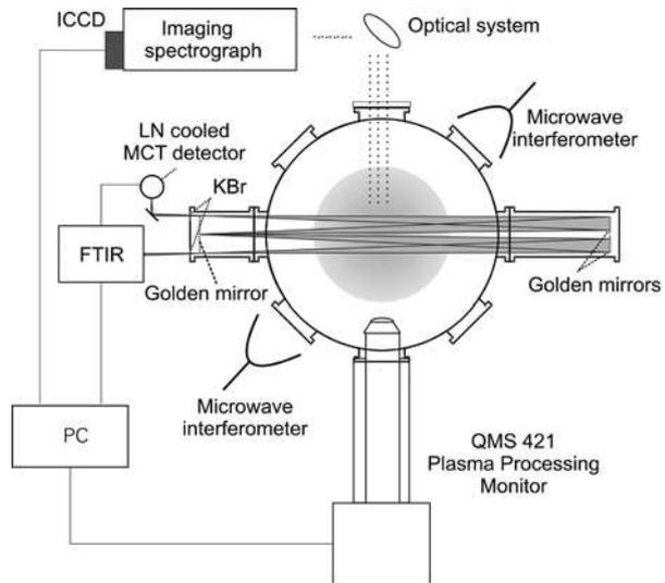
**Fig. 1.** *Experimental set-up, top view. For the more detailed explanation and abbreviations see text.*
