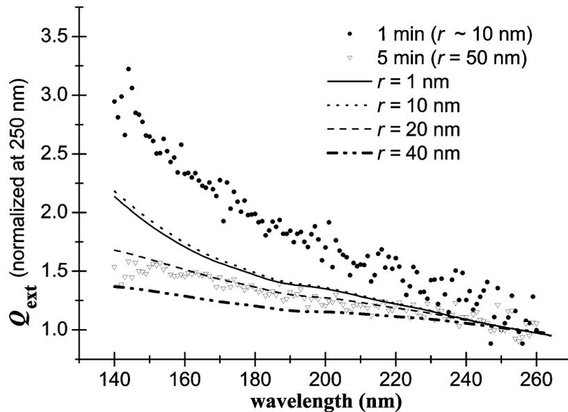
**Fig. 4.** Comparison of calculated and measured UV extinction curves for different particle radius: solid lines - calculated curves for ACH2 material according to Bohren and Huffman (1983) with  $Q_{ext}$  from Zubko et al. (1996); symbols - measurement results.
