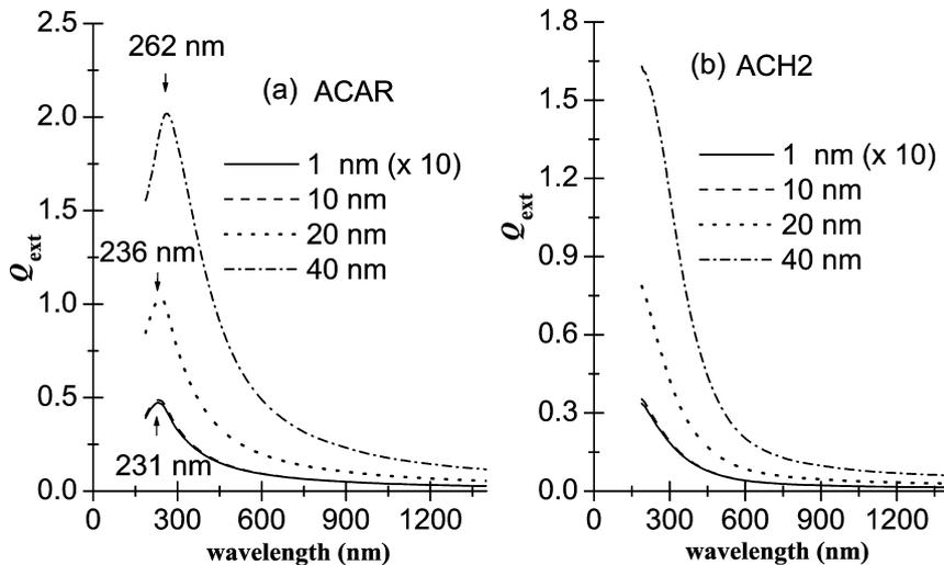
**Fig. 3.** Extinction curves for different particle radii. The refractive index necessary for the calculation of  $Q_{\text{ext}}$  was taken from Zubko et al. (1996): (a) low-hydrogenized material, graphitic-like (ACAR); (b) hydrogen-rich material, polymer-like (ACH2).
