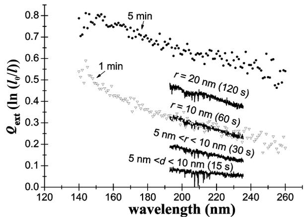
**Fig. 2.** Extinction curves ( $Q_{ext}$ ) for different particle radii (different discharge times). UV extinction curves are measured with two different spectrographs/detecting systems: solid lines - extinction measured with UV/VIS spectrograph and ICCD; solid circles and opened triangles - extinction curves for extended spectral region (VUV).
